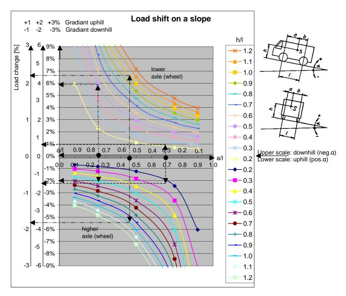
Weight differences in relation to the actual axle and wheel load at gradients of 1%, 2% and 3%
